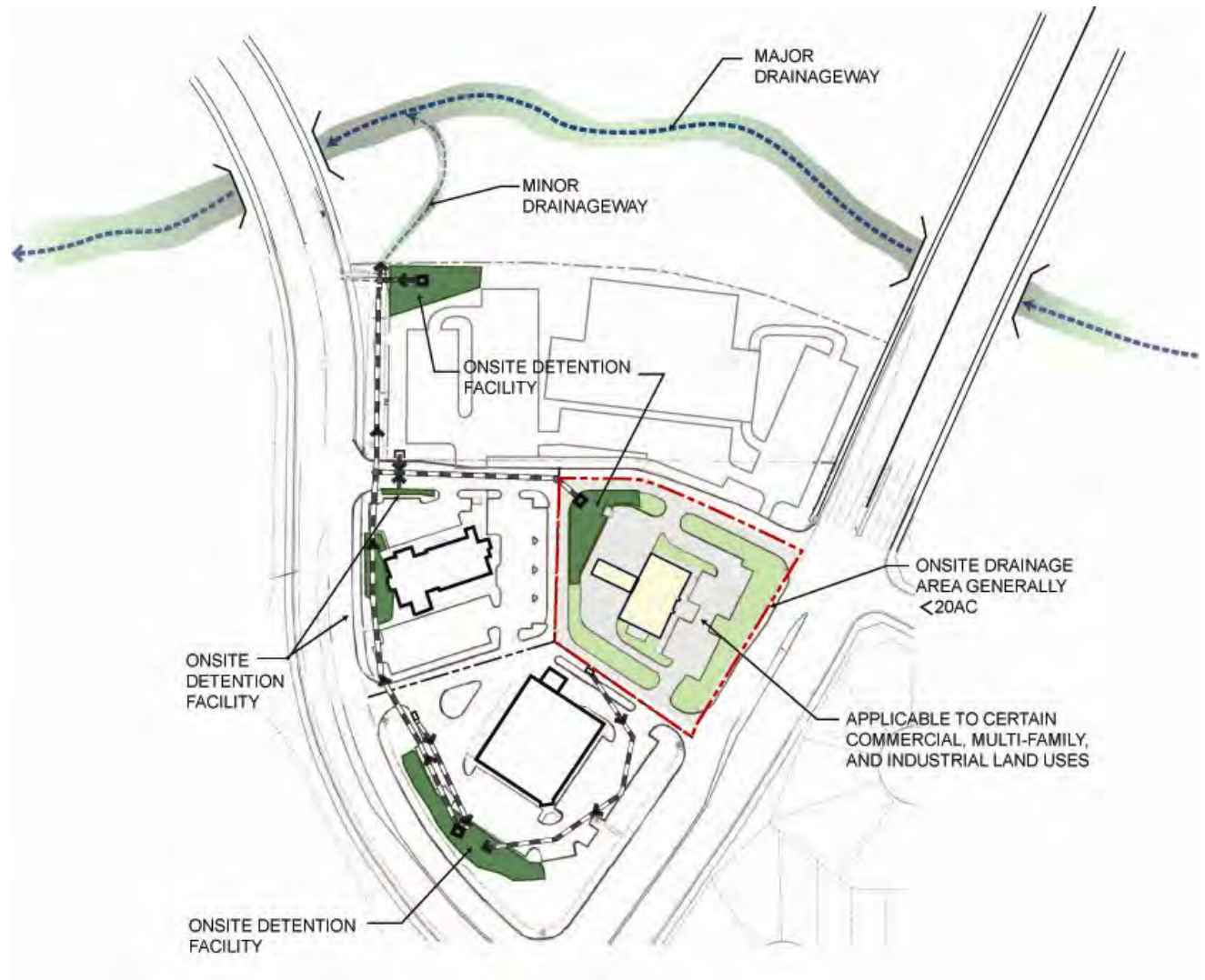
FIGURE 13-4 ONSITE DETENTION APPROACH
